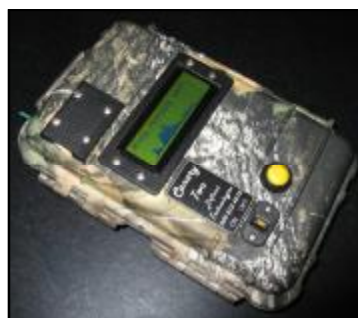
Figure 3: Above is the gas module used to collect the data shown in figures 1 and 2. This module uses 2 SAW detectors; one in the bypass collection sample train and one in the GC analysis train.
