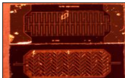
Figure 1: 11ppbv methyl mercaptan retained on a modified PDMS stationary phase.
