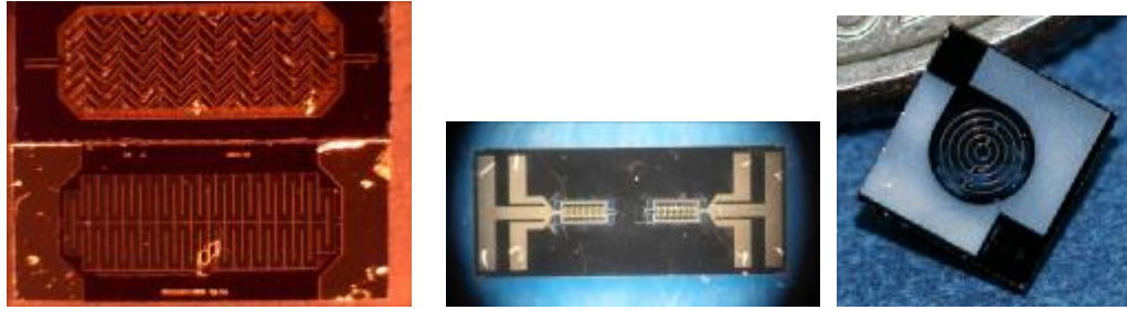
Fig. 4a. (left) high surface area tortuous path preconcentrator (TP-PC) 4b. (center) low mass pivot plate preconcentrator (PP-PC) 4c. (left) concentric ring preconcentrator (CR-PC)
