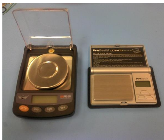
Figure 3: These are two portable balances that would be suitable for use in the field. It is suggested to use a balance that can read to 0.01 g.
