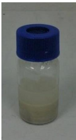
Figure 2: This is a 20mL VOA vial containing our soil sample and the methanol used to extract it.
