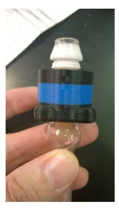
The pictures on the left and right show the proper installation of the sparge bottle ferrule. On the left the ferrule is show on a globe neck sparge bottle. On the right, it is shown installed on an air sample adapter.
