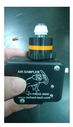
If your retention times aren't lining up correctly or you cannot get a consistent calibration. First inspect the sparge bottle ferrule. If it is improperly installed, it can create a small leak in the system and cause this variation.
