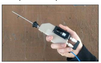
The Inline Diluter provides a convenient way to dilute high concentration air samples
